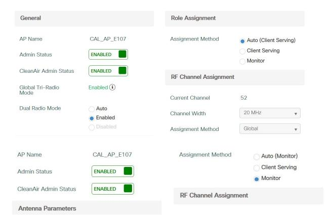
Here is tri radio in action, with slot 0 (2.4GHz) serving clients on channel 1, slot 1 (5GHz) serving clients on channel 52, and slot2 used for dedicated monitor mode.
